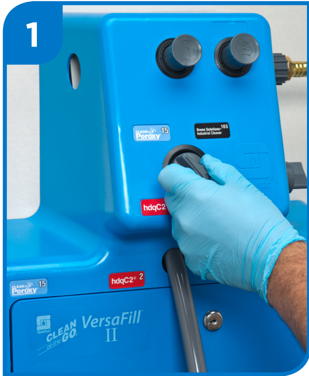
Select bottle fill product by turning dial to desired product
