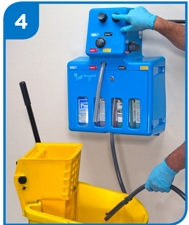
Push right button for bucket fill
