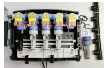
4) Unscrew Eductor and Inspect
