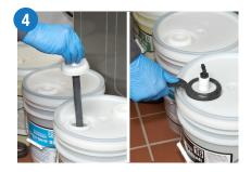
Insert 3/8" barbed insert (964900 [5gal.], 965700 [15gal.], 965900 [30gal.], 967500 [55 gal.]) or tube stiffener into the container and secure properly.
