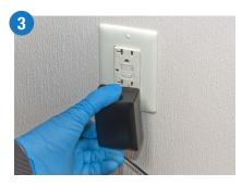
Connect the wall power adapter to a wall outlet providing 110V to 240V AC at 50 - 60 Hz to 0.8 amps.
