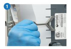
Use cover key to open cabinet. Push key into the center slots on the right side to release, then lift cover.
