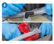
Measure and cut outlet tubing to the desired length.
