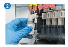
Insert the white flush vent valve into the first eductor (left-most eductor). Do not connect any chemical hoses to this valve.
