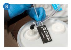
Affix line tags at the bucket and below the check valve to identify chemical being dispensed.
