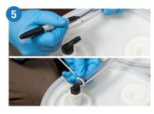
Measure and cut 3/8" x 5/8" vinyl tubing (961700) to the length needed to connect the containers to the dispenser check valves. Then, connect and secure the tubing to the barbed inserts.
