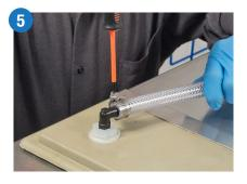
Attach outlet tubing to the washer where appropriate.
