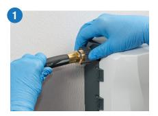
Connect incoming water supply using fittings provided. This will either be a 3/4" female garden hose or a 1/2" O.D. push-fit connector. Use 1/2" braided tubing (964800) when creating your own water manifold system.
