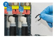
Insert check valve elbow into the appropriate eductor, secure with clip.
